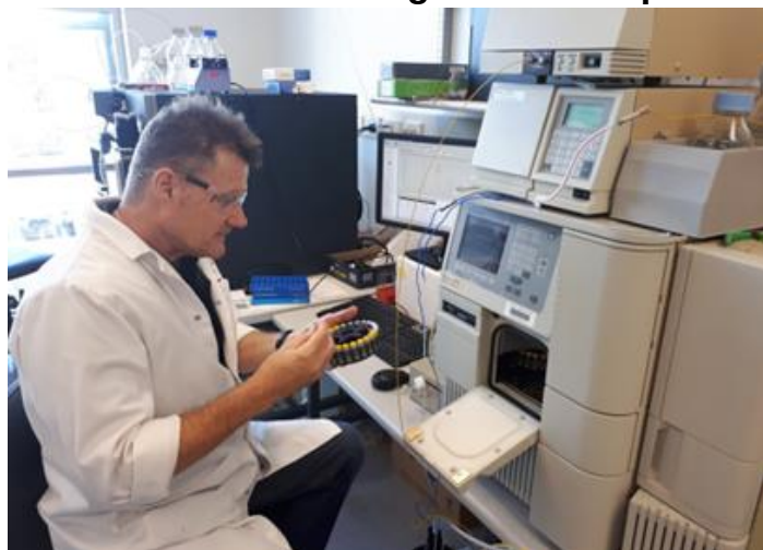
Figure 11 Measuring simple sugars by High Pressure Liquid Chromatography with Refractive index detection (HPLC-RI).
