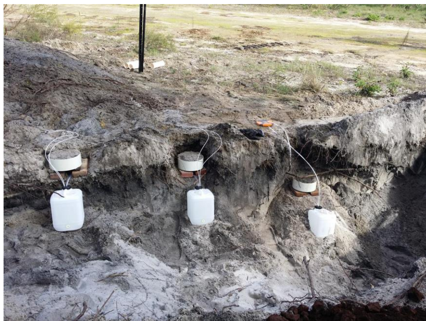
Figure 6: Layout of small plot in the Wanneroo field trial. The plot has three lysimeters at varying depths.
